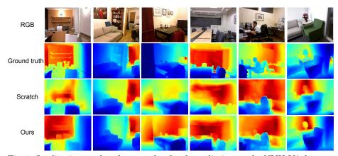
Fig. 1: Qualitative results of monocular depth prediction on the NYU-V2 dataset.
