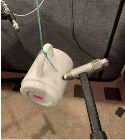
**Figure 6:** Physical setup for Analysis by Synthesis dataset collection. A microphone at the top left records audio from the suspended ceramic mug being struck by the impact hammer on the right.
