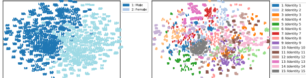
Figure 4: Our learned cross-modal embeddings of voices for 15 speakers from the VoxCeleb1 test set visualized with t-SNE. The two figures are color coded with gender and identity, respectively.
